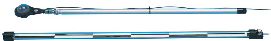
Solar radiation sensors (from top) Dome Net Radiometer NR2 and Tube Solarimeter TSL
