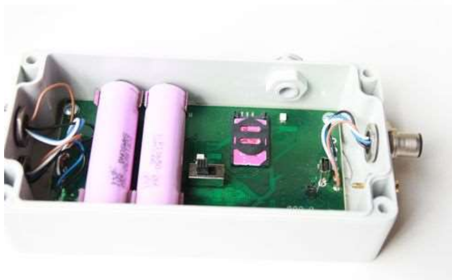
Obr. 6: slotu pro SIM
