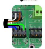
In DeltaLINK configure channel 1 - 6 as Moisture Probe SM150T and channel 7 as SM150T Temperature.
