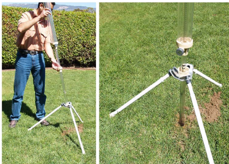
Fig. 24. Left: lowering GP into Tripod and Borehole.
