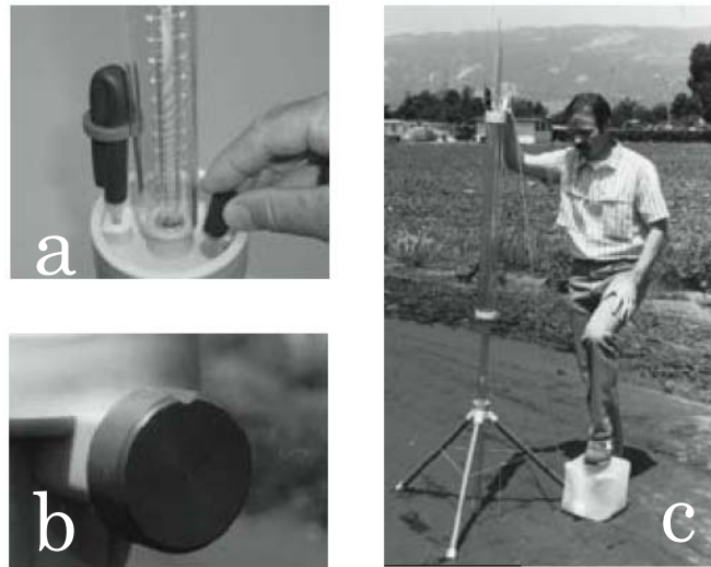
Fig. 28 - Filling the Reservoir with water using the collapsible water reservoir.
