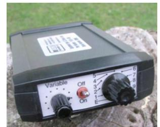
The PLU5 can be used to maintain a single constant light concentration within the leaf chamber or be used to generate data for rudimental A/Q (light response) curves.
