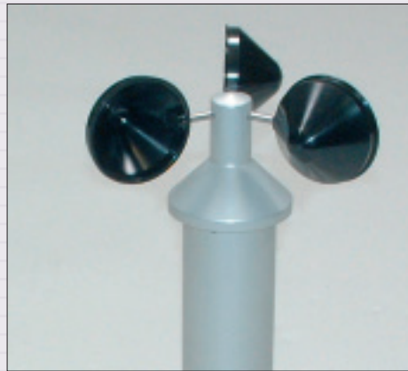
Wind speed sensor (16.98.50)
