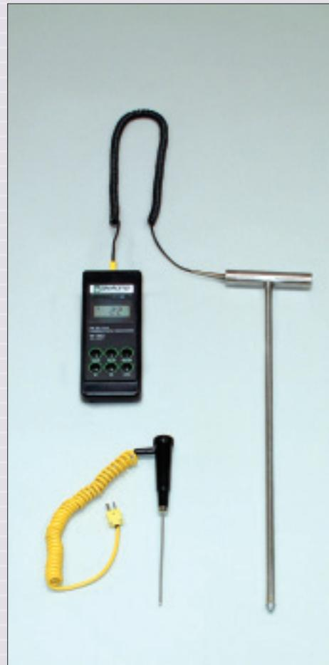
Digital thermometer with compost temperature probe
