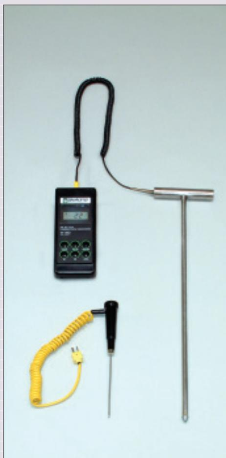
Digital thermometer with compost temperature probe
