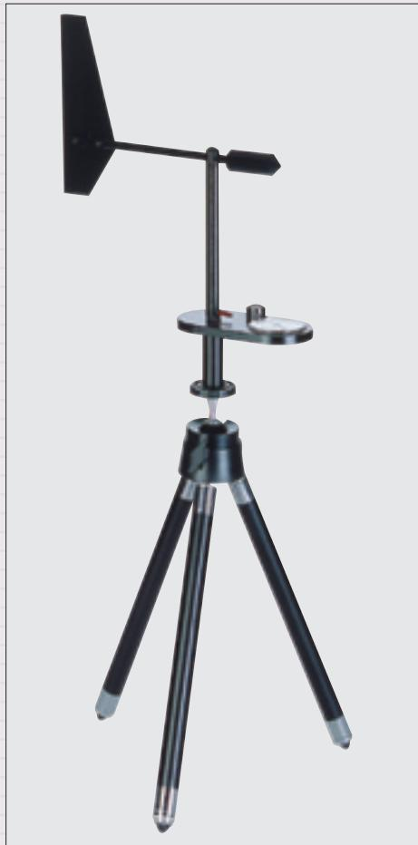
Wind vane with tripod
