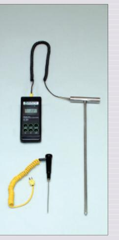
Digital thermometer with compost temperature probe The thermometer can be used to measure temperature in degrees Celsius and Fahrenheit and has a measuring range of -50 tot +150°C. Accuracy is 0.5°C. The display can be read to 0.1°C. The thermometer has options to display the measurement and to reset the maximum- and minimum temperature and hold facility. Power supply four 1.5 V AAA batteries.
