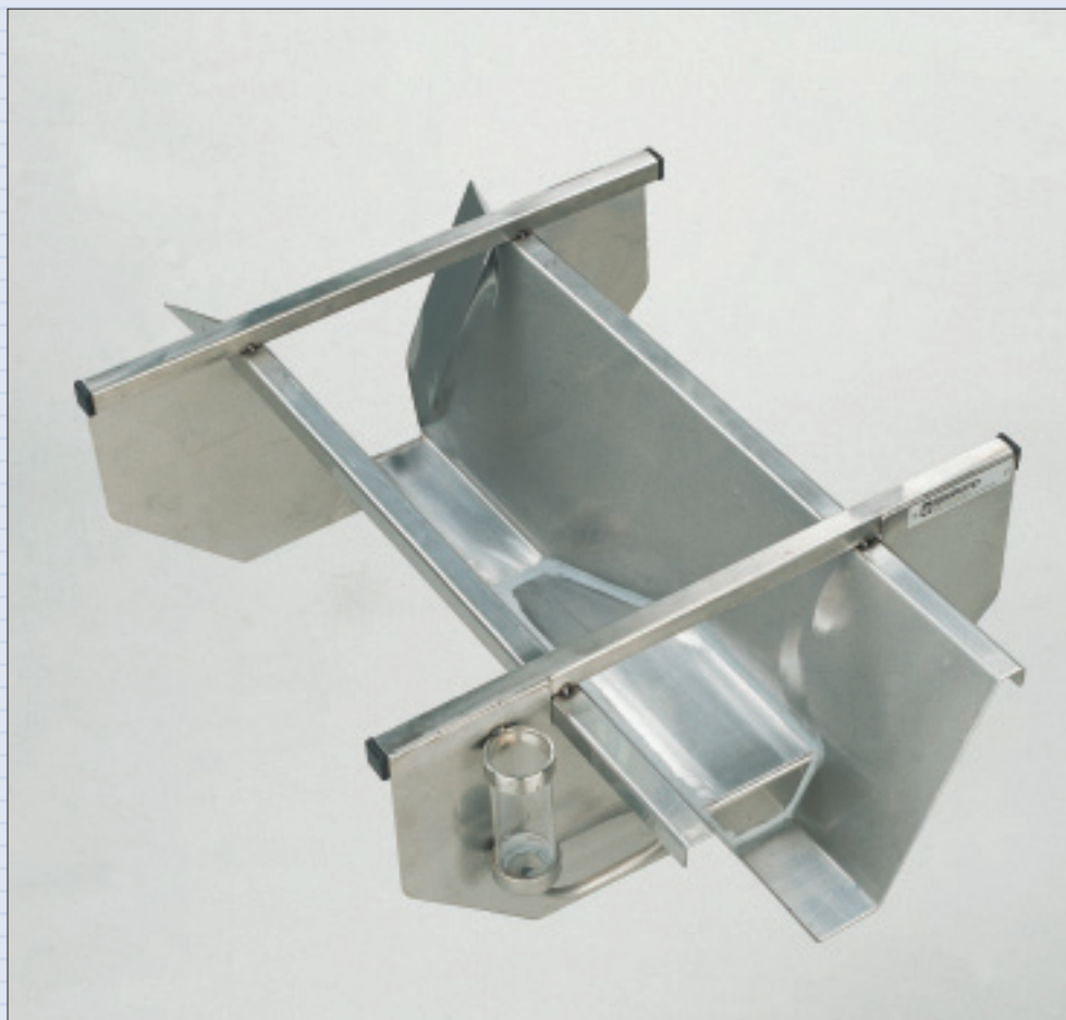
Small RBC flume for manual read-out
