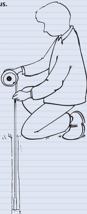
Measuring the water level with the sounding apparatus provided with a frame, in deeper monitoring wells.
