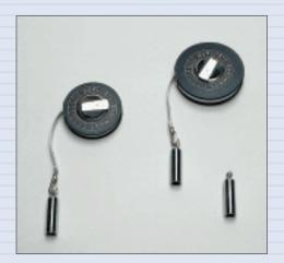
Measuring tapes with sounding device
