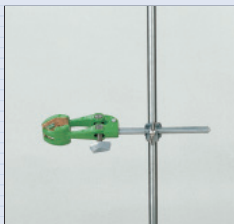
Third hand to hold sample flasks
