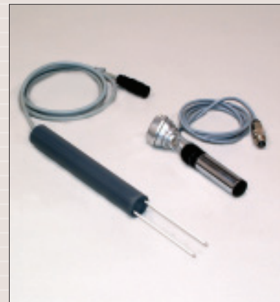
Tensiometer and soil moisture sensor
