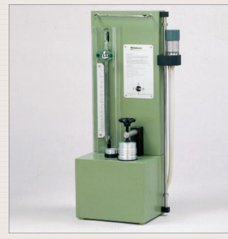
Air pycnometer according to Langer
