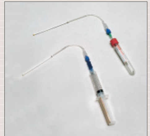
Rhizon with vacuum tube and syringe
