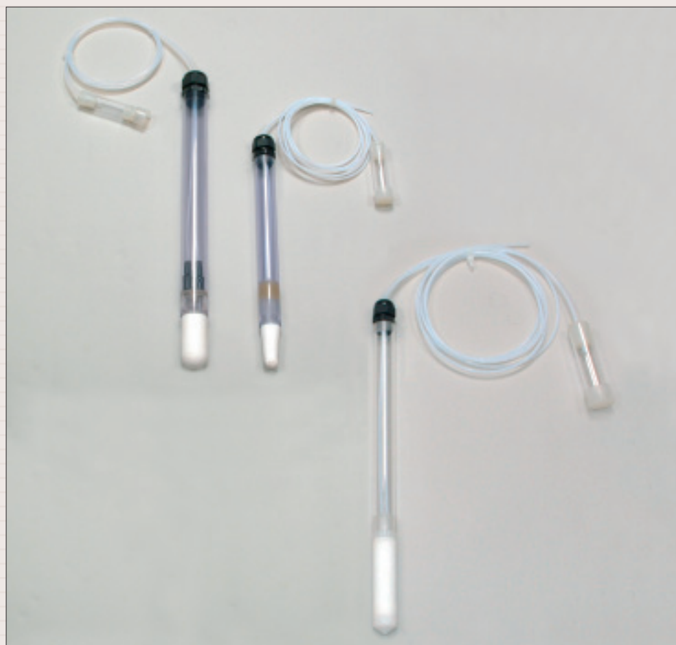
Soil water samplers with glass and plastic porous cup
