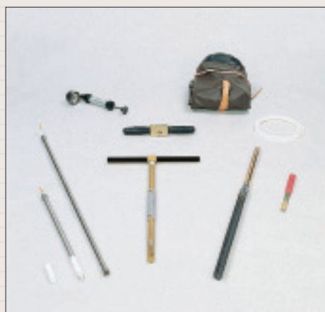
Soil moisture sampling system (SA)
