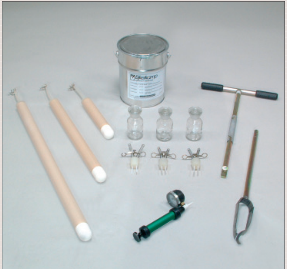
Soil moisture samplers with large ceramic cup, standard set
