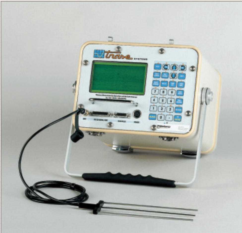
Trase soil moisture measuring system
