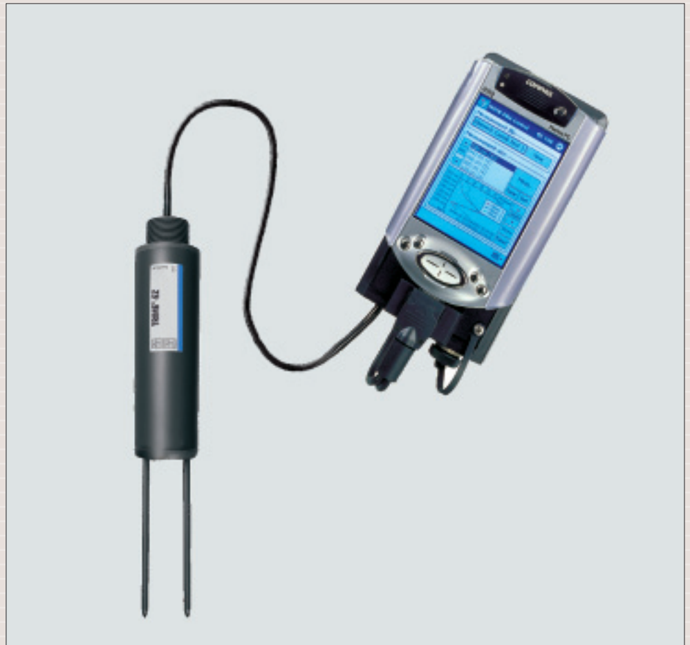
Trime Data Pilot system connected to intelligent (stand alone) probe
