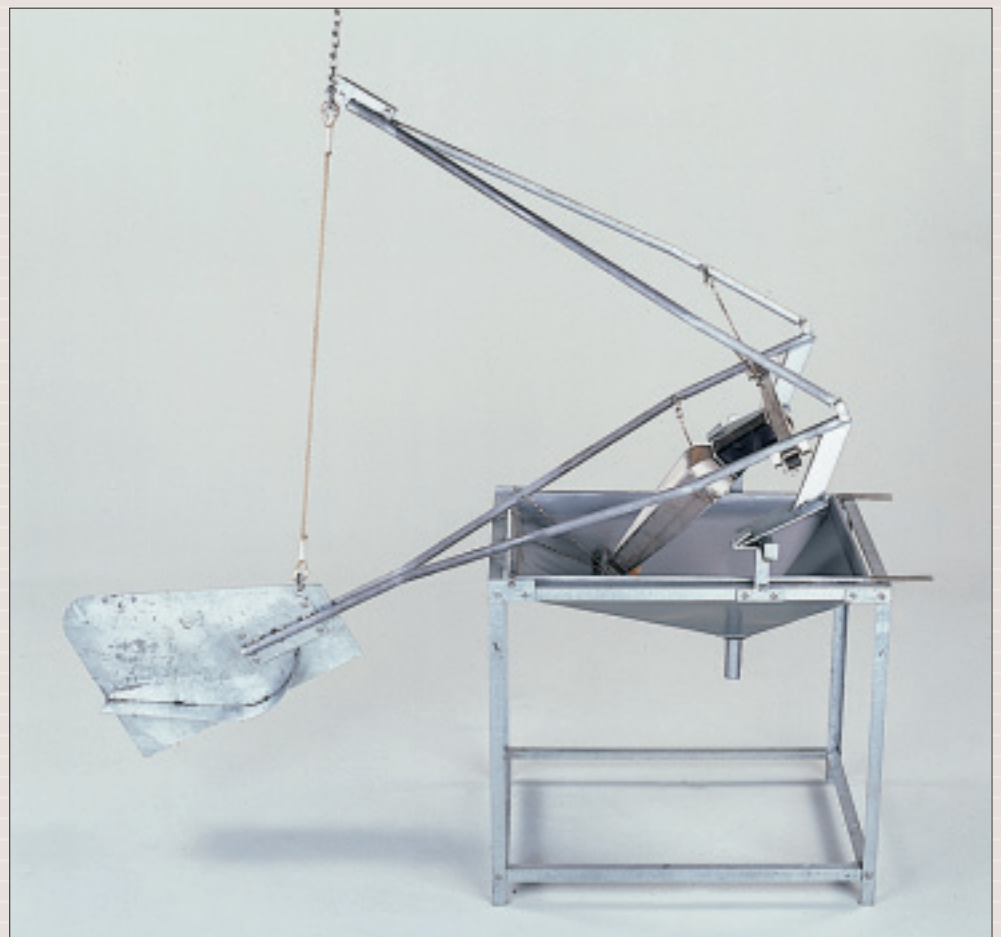
Bed load transport meter, Arnhem type
