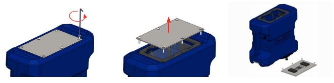
2.1.2 Disconnecting the power cables and connecting the battery
