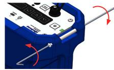
2. Remove the carrying strap pin by pressing it out of the housing chamber with the hex key. Push the pin out of the hole until it reaches the position shown.
