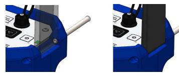
4. Push the carrying strap pin back into position using the hex key, while twisting clockwise if necessary.
