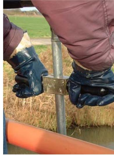
Dismantle the extension rods two by two if necessary. If you shake the rods backwards and forwards slightly, the screw connections will generally become loose. You can leave one extension rod in place without causing problems. "Row" the sampler through the water a few times to rinse it off as much as possible. Bring it on board or to the water's edge.
