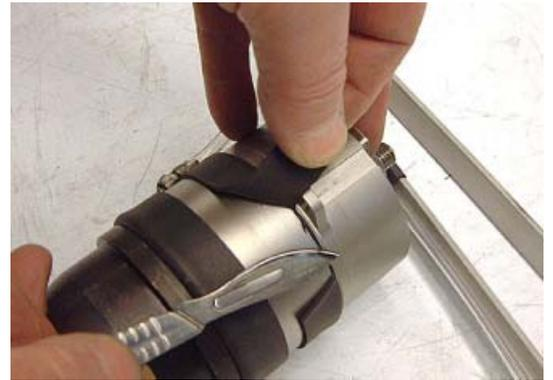
Push the ring with clamping pins over the cutting ring and fit the new nuts that are included in the set by hand. Tighten the nuts **alternately and a little further each time** using the box spanner. After that, you can remove the clamping tool and fit the cutting head back into the frame.
