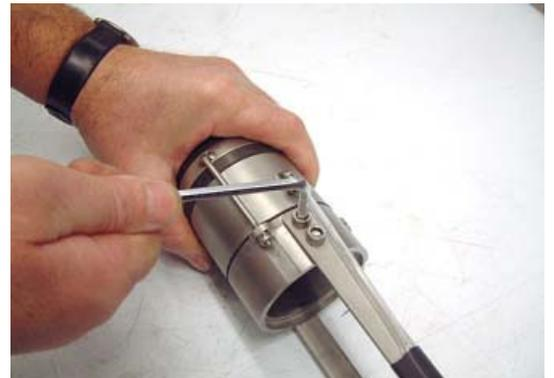
Take the cutting head and the small box spanner from the tool set. Remove the three nuts from the cutting head by loosening all three slightly first and then unscrewing them further. Remove the ring with the threaded pins, the upper collar, the cutting ring and the damaged membrane.
