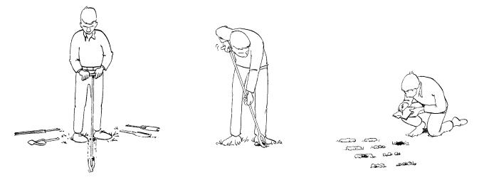
1. Hold the Edelman auger by its handle and rest it on the ground. Using some pressure, rotate the auger clockwise into the soil. After approximately 2¼ full turns (of 360°) the auger will have bored itself 10 cm into the ground. The auger will then be filled up to the bracket with slightly disturbed soil material. Dependent on the type of soil it requires more or less turns to fill the auger.
