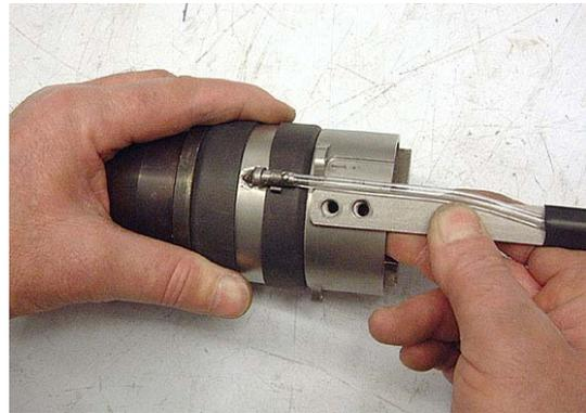
Place the crosspiece of the clamping tool in position and fit the ring and swivel. Make sure all the parts are properly centred and check this when tightening the swivel. Everything must now be clamped together tightly using the clamping tool. Use a spanner if necessary.
