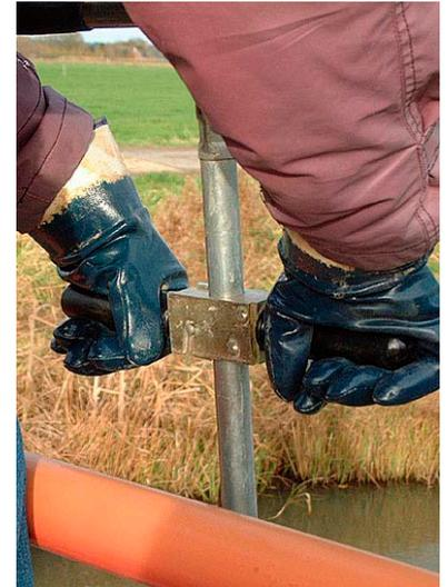
Dismantle the extension rods two by two if necessary. If you shake the rods backwards and forwards slightly, the screw connections will generally become loose. You can leave one extension rod in place without causing problems. "Row" the sampler through the water a few times to rinse it off as much as possible. Bring it on board or to the water's edge.
