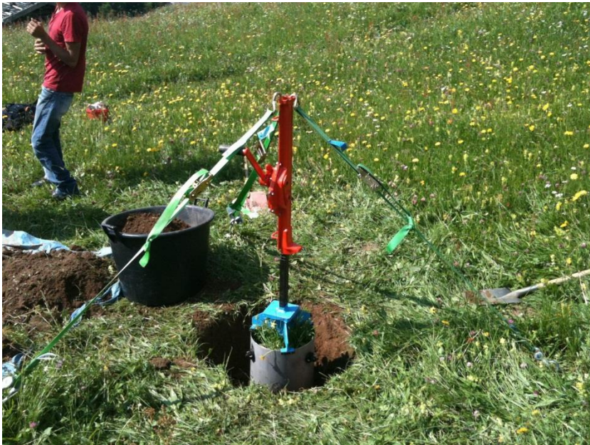
Soil column cutting with jack lift device
