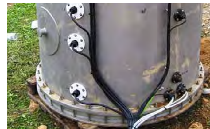
The lower part of a Science-Lysimeter just equipped with instruments
