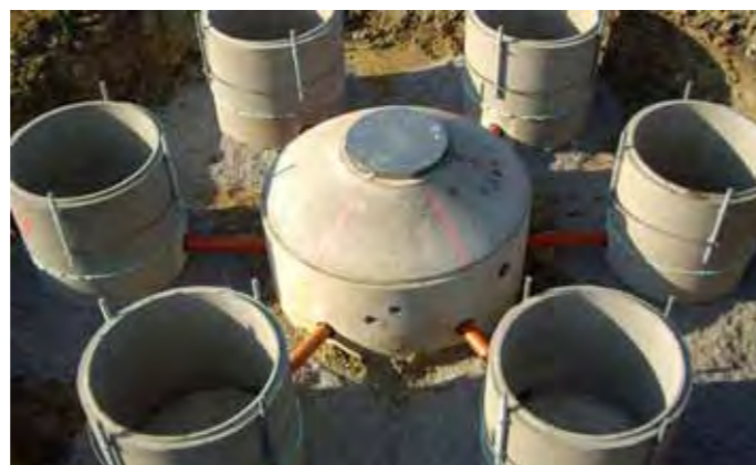
When completely surrounded by the field's soil the Lysimeter obtains a field-identical temperature profile
