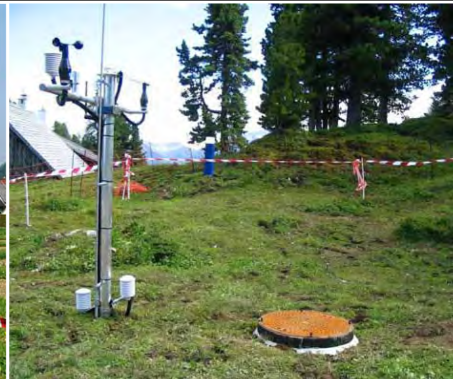
Customized weather station with Lysimeter (between trees and access hatch)
