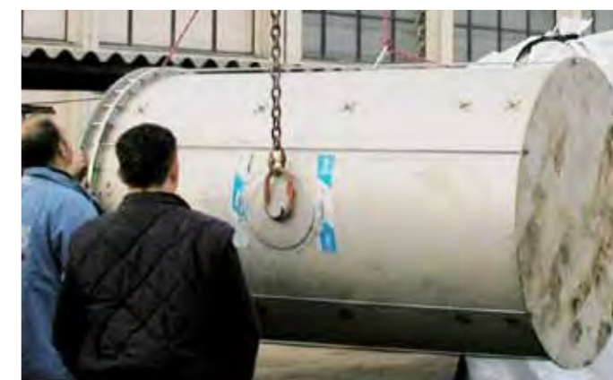
Safe rotation of the Lysimeter without deformation
