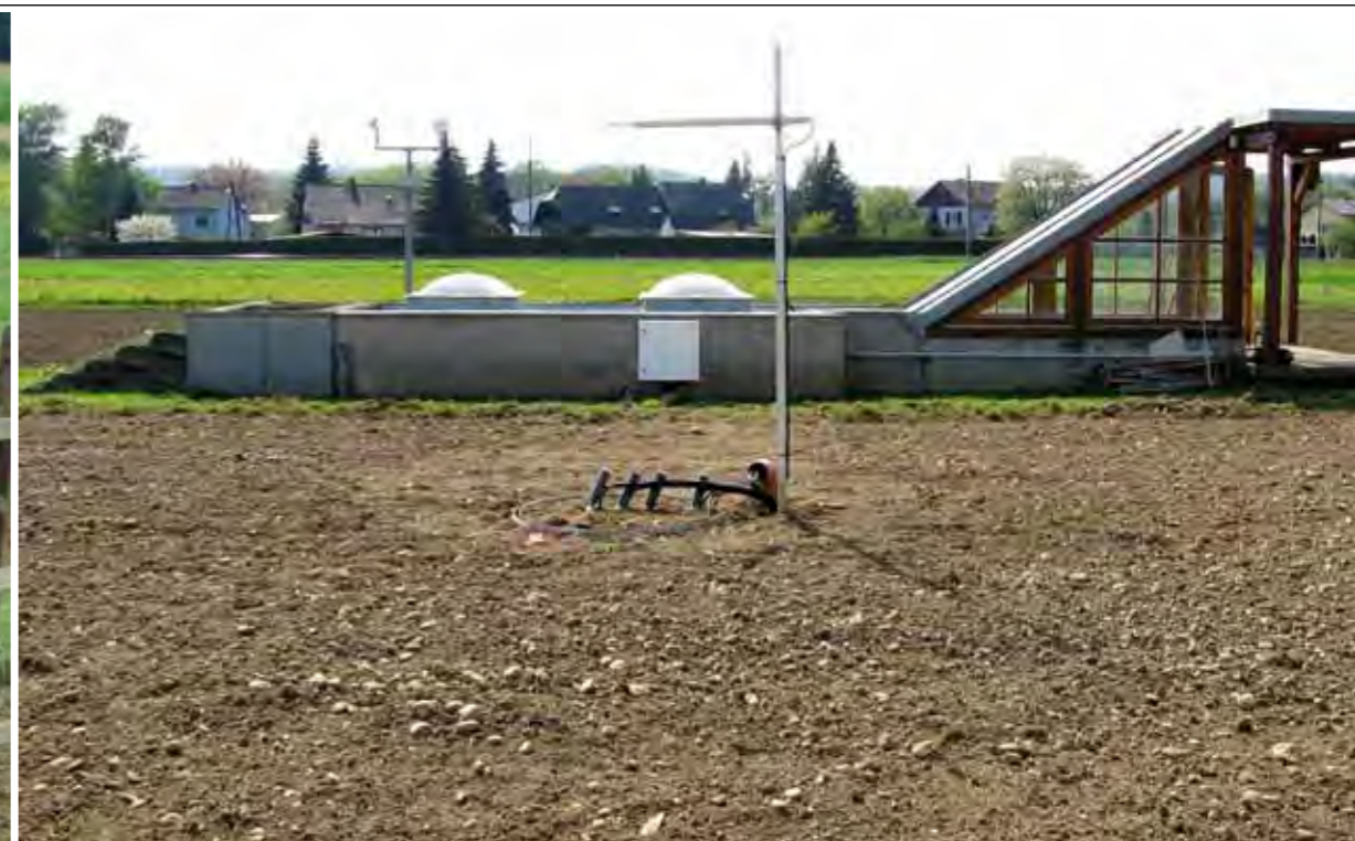
Field with Agro-Lysimeter after sowing
