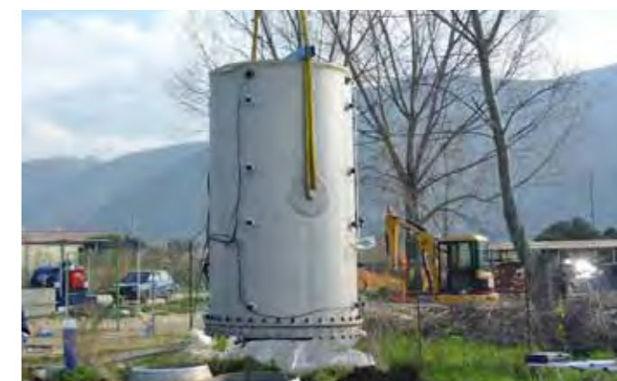
Safe lifting of a Lysimeter with a weight of a few tons
