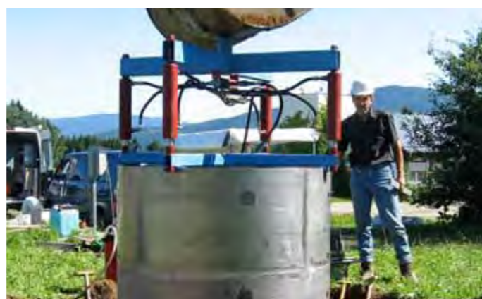
The quadruple hydraulic press in action
