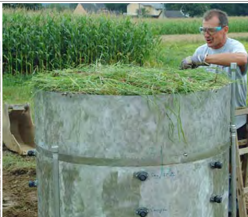
Agro-Lysimeter with removable cylinder section
