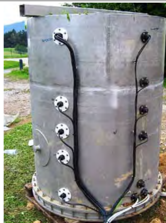
Lysimeter with installed sensors
