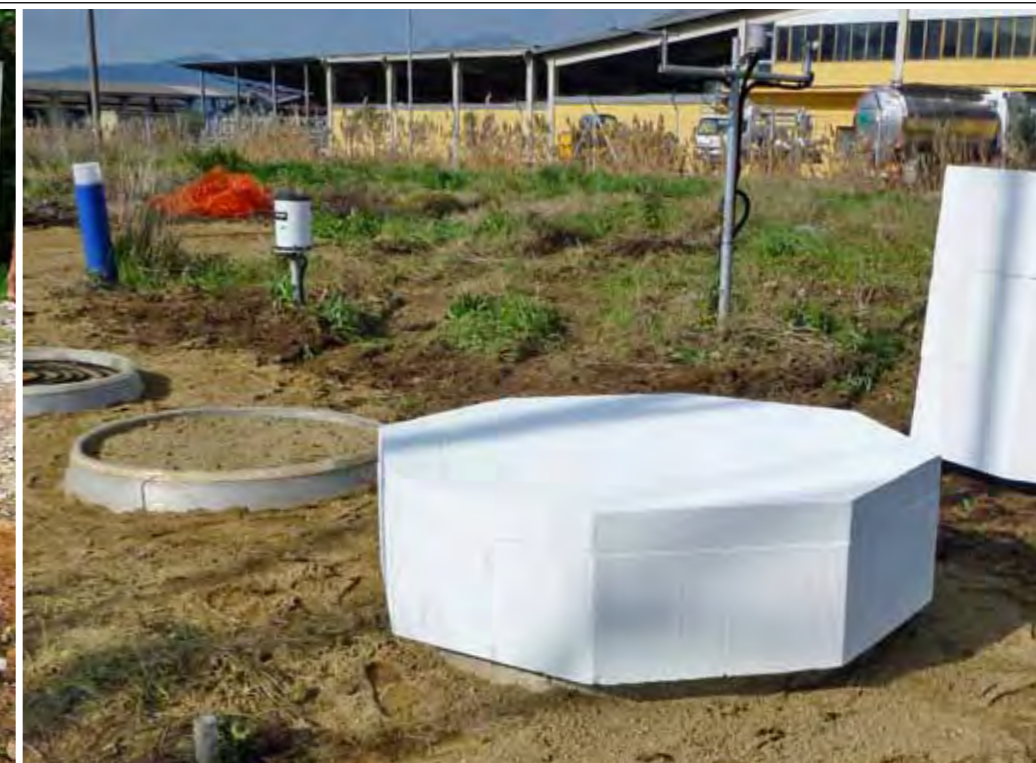
Science-Lysimeter with climate chamber
