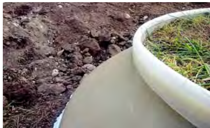
A installed sealing lip on a Hydro-Lysimeter just being prepared
