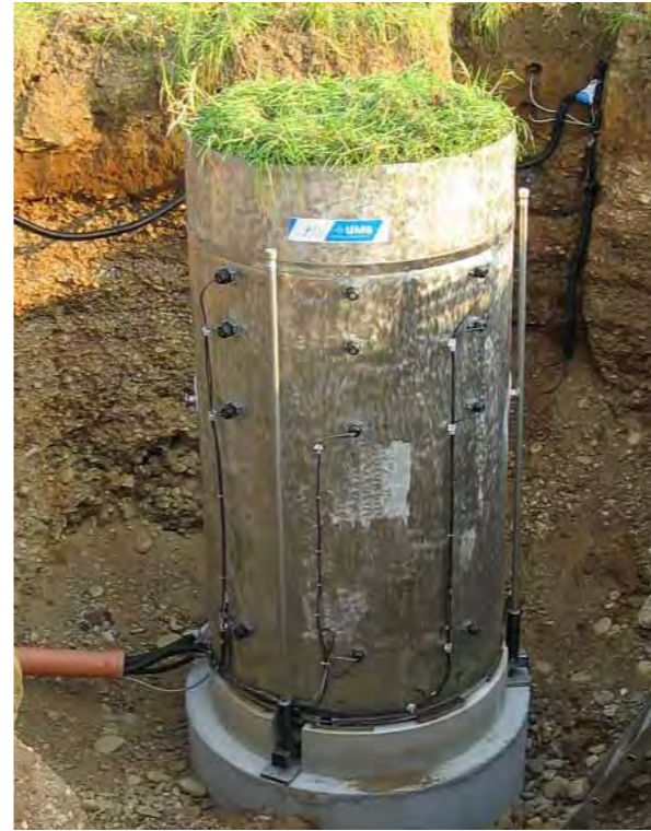
Lysimeter with installed sensors, field sensors in the background
