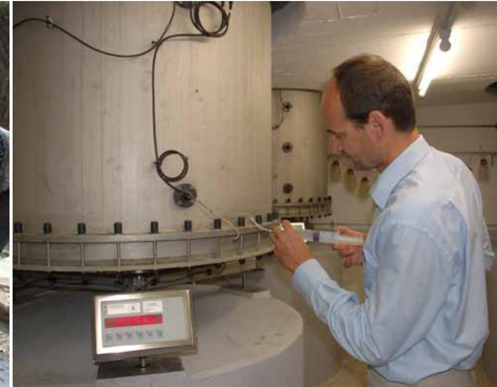
Refilling of a tensiometer with filling syringe
