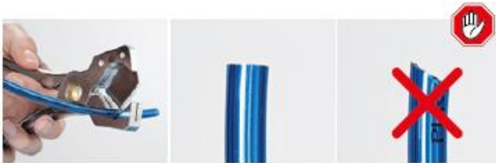
Figure 28: cutting the tubes correctly
