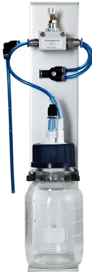
Figure 8: apparatus for aliquot sample taking
