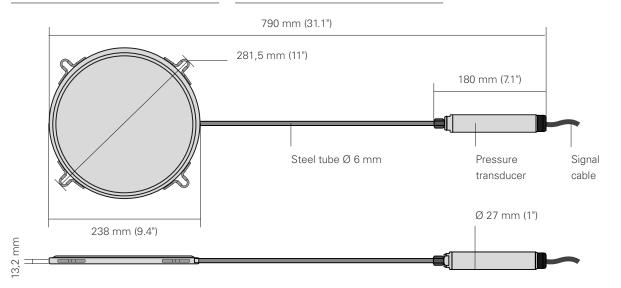
WWW.SISGEO.COM EARTH PRESSURE CELLS 3
