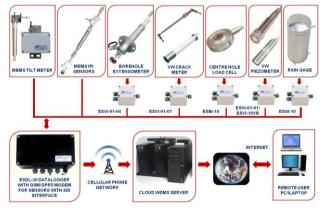
connect the sensors to the datalogger. The beauty of the system is that only а single 3 conductor cable is required to interconnect all the sensors and the datalogger in a serial bus. SDI-12
