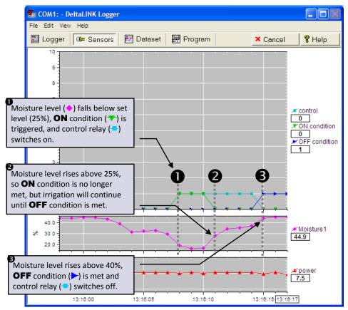
**Note**: you should be able to hear the GP1 relay switching, but it may be convenient to attach a multi-meter to the end of the control cable, so that you can check the switching remotely.
