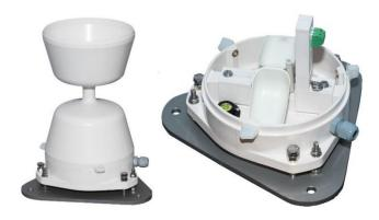
Traditional cylinder-shaped rain gauges are inaccurate due to the effect of wind blowing over the orifice. The physical presence of the gauge causes air to accelerate, carrying rainfall away from the collecting vessel. The effect of this can be up to a 20% reduction in rainfall catch. The unique aerodynamic shape of the EML range of scientific standard rain gauges reduces this effect, ensuring a high level of confidence in the accuracy of our measurements.
