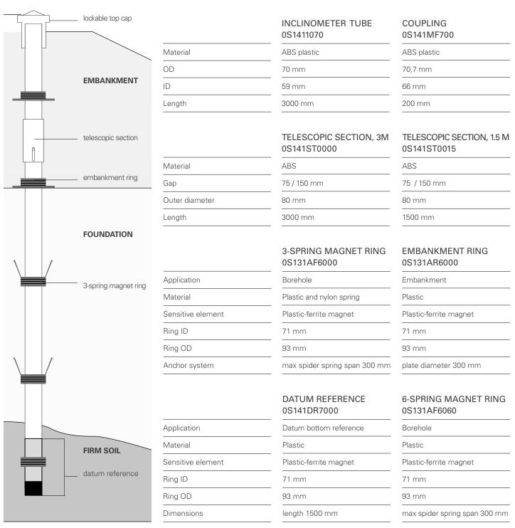
WWW.SISGEO.COM MAGNET EXTENSOMETER 4
