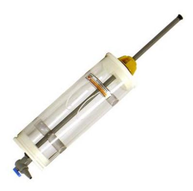
The Kemmerer water sampler (vertical water bottle) is used for general water sampling in lakes, channels, wells and the sea. This sampler consists entirely out of plastic parts so that there is no risk of the sample coming into contact with metal. The transparent acrylic bottle body allows viewing your sample before removal. A thermometer can be mounted inside acrylic Kemmerer bottles. The standard Kemmerer water sampler holds 1.2 litre.
