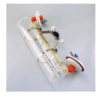
Intended for shallow or deep open waters, these bottles are called "horizontal" because they descend, parallel to the bottom. They are pulled sideways just before closing by the operator. This ensures a representative water sample for that specific depth. They are ideal for sampling at the thermocline, at other stratification levels, or just above the bottom sediments.
