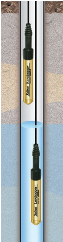
Figure 1-5 Levelogger and Barologger in Well
