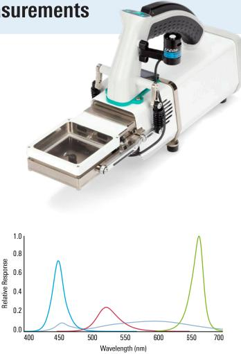
**Figure 7.** The large light source provides peak emission at 453 nm for blue, 523 nm for green, 660 nm for red. White is nominally at a 4000 K color temperature.
