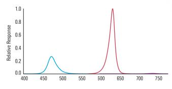
Figure 2. The 6800-01A fluorometer peak outputs are at 475 nm for blue, 625 nm for red modulating and actinic, and 735 nm for far-red.
