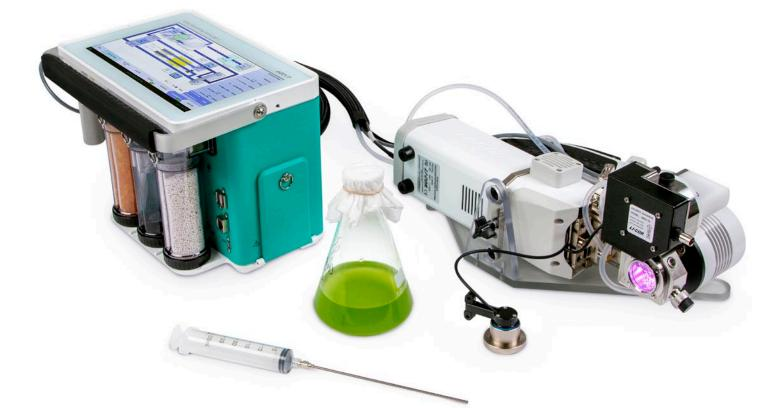
The Aquatic Chamber (6800-18) provides measurements of  $CO_2$  exchange and chlorophyll *a* fluorescence from samples in liquid water, such as algal suspensions, or samples that require high ambient humidity, such as bryophytes. Assimilation is computed from the concentration differences and flow rate
