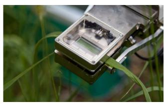
The Clear-top Chamber (6800-12A) is compatible with the small light source.
