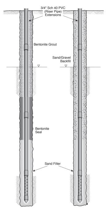
Typical Standpipe Piezometer Installations
