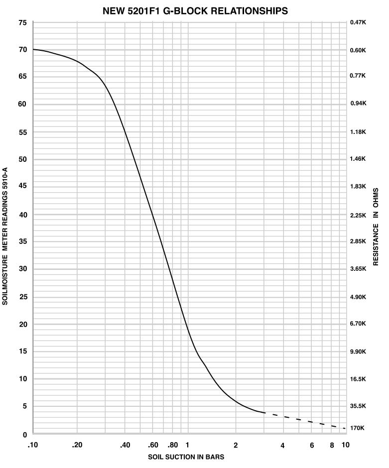
The relationship between Soilmoisture Meter readings and impedance in Ohms is based on a 350 mV step pulse having a frequency of approximately 60 cycles/second. The impedance values in Ohms, as shown, represent a signal/response relationship and that may vary with alternative sources of signal excitation.
