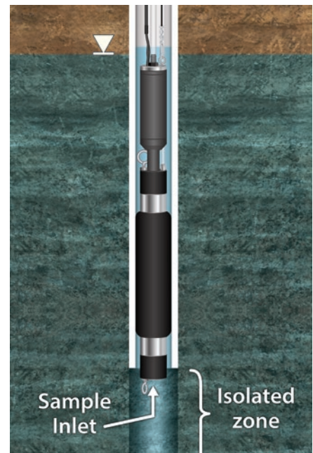
A Model 800M Packer can be used to isolate the sampling zone and reduce purge volumes.
