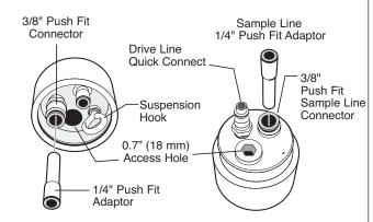
Wellheads come with two Push Fit Adaptors so that either 1/4" or 3/8" tubing can be used, as preferred.
