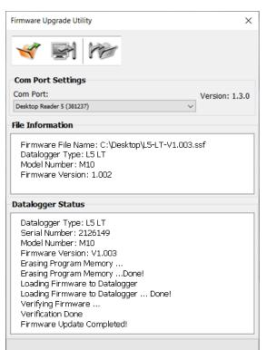
6) If, however, a communication error occurs between the "Verifying Firmware" and the "Loading Firmware to Datalogger" messages, then please contact Solinst. You will need to give the datalogger Serial Number and explain the exact positioning of the error message.
