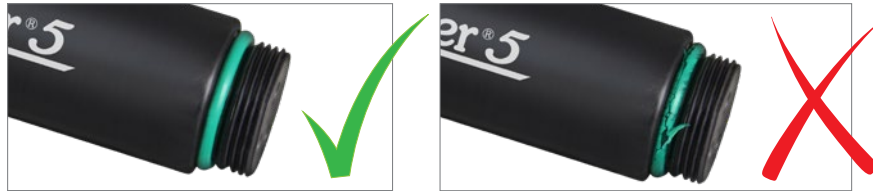
Figure 10-25 Levellogger O-ring Damage
