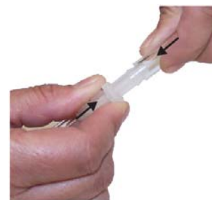
Fig. 13. connecting two pieces of tubing using a Tubing Coupler.
