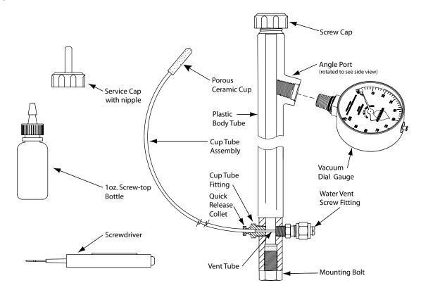
(Figure 2) - 2100F Soilmoisture Probe Parts
