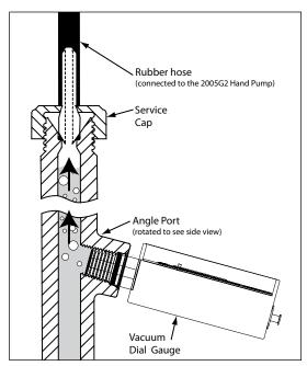
(Fig. 6) Removing the air from the probe with the 2005G2 Vaccum Pump
