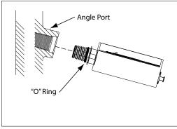
(Fig. 4) Attaching the dial gauge
