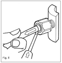
(Fig. 9) Replacing the cup tube
