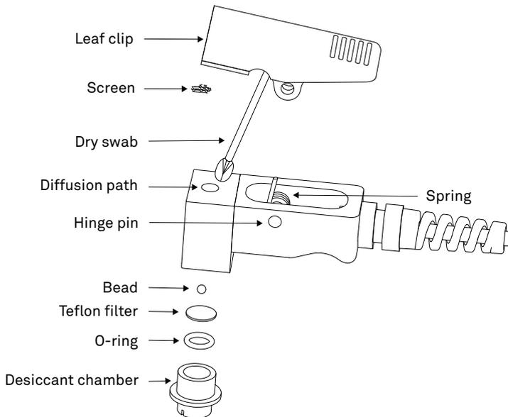
Figure 56 Thorough cleaning of the diffusion path
