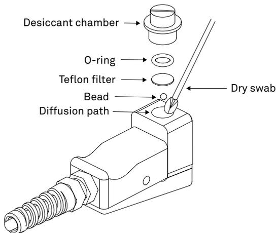
**Figure 55 Quick cleaning of the diffusion path**
