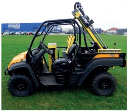
The **Wintex MCL3** is developed for intensive use in the work involved in measuring the remaining content of nitrate in the soil. Soil sampling is conducted from the control panel and is carried out by a hydraulic system. The control panel has four functions:
