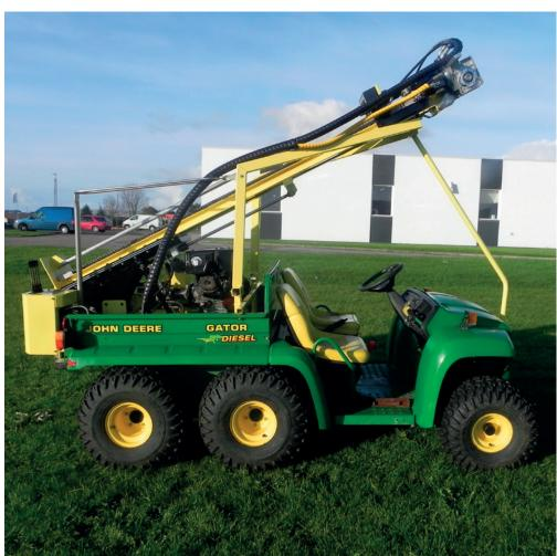
The **WINTEX MCL3** is an extremely robust soil sampler which takes soil samples in any kind of soil, also in very hard soils. Its ability of operating in all kinds of ground as well as the high quality of the samples has led to the WINTEX MCL3 being the leading soil sampler for samples up to 120 or 200 cm.
