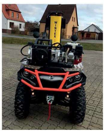
The **WINTEX 3000** is an efficient and strong automatic soil sampler. It is user-friendly, easy to use and requires only minimum maintenance. All functions are easily carried out from the driver's seat.
