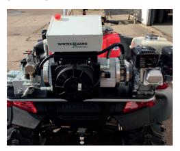
The custom-made oil tank is made of aluminum. It has a ribbed surface which means that its area is three times larger than a plain surface. Because of the aluminum and the ribbed surface the cooling capacity is 12 times higher than the cooling capacity of a traditional oil tank. This means that the tank ensures optimal cooling of the hydraulic oil.
