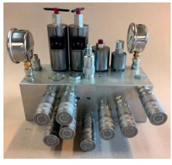
All functions are carried out from the distribution block which is custommade. The hydraulic system has a simple construction which makes it easy to maintain.
