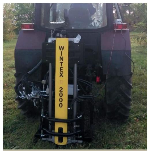
The **WINTEX 2000** can be mounted on all vehicles including pick-ups, tractors and trailers.
