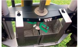
Soil from different layers is automatically filled into two soil boxes. Dividing the samples is conducted with close accuracy.
