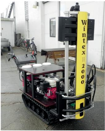
The **WINTEX 2000** is an efficient and strong fully automatic soil sampler. It is user-friendly, easy to use and requires only minimum maintenance. All functions are comfortably carried out from the driver's seat.
