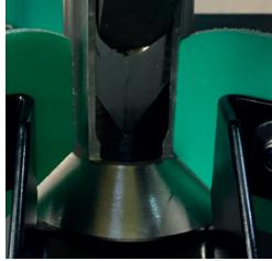
The scraper precisely fits the inner diameter of the probe, and the scraper blades ensure that the probe is emptied fully before going into the ground again.
