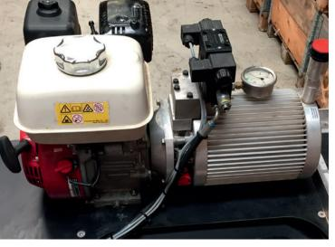
The hydraulic system is custom-made to fit the **WINTEX 1000** and is mounted on a robust and strong Honda GX160 motor.
