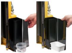
The **WINTEX 1000** is available with different holding boxes which fit most of the commonly available sample boxes or with a holding box from which the sample can be filled directly into a soil bag.
