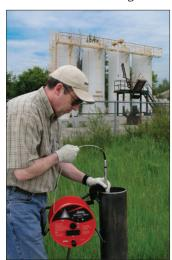
oil/product the signals are steady. If the liquid is water (conductive liquid greater than 50 µS/cm), the conductivity of the water completes a conductivity circuit. This overrides the infra-red circuit, and the tone and light are intermittent.
