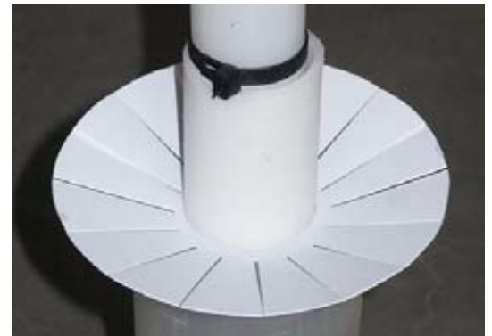
Fig. 15 Catcher localized with tie rib
