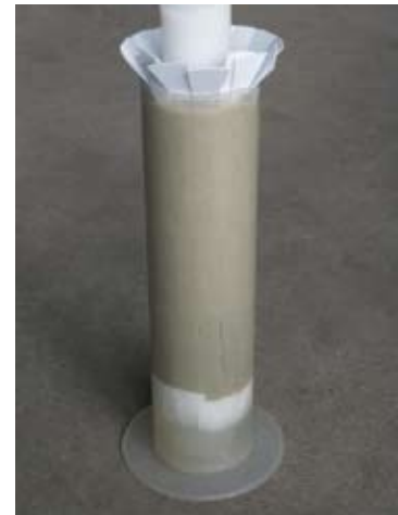
Fig. 19 Bentonite fully swollen
