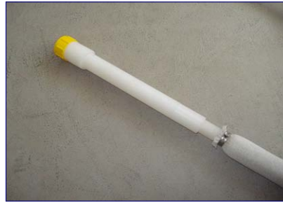
Mini pre-packed monitoring well with filter sand pre-packed in tight-fitting filter gauze (right) with riser pipe 18.2x26.6 mm with coupler and top cap
