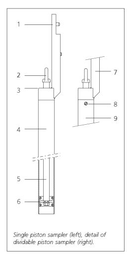
The piston samplers of both sets are fitted with a bayonet connection (1) to which extension rods can be attached. It is welded on the outside to permit free passage of the extension rod.
